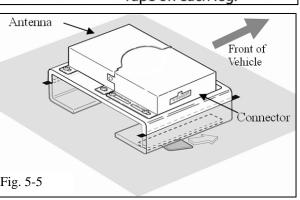
(1) Make sure the bracket is firmly attached to the floor pan by firmly applying pressure down on the receiver/bracket assembly.
