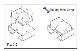
(b) Install the receiver onto the bracket using the eight (8) screws supplied in the kit. (Fig. 5-2)
