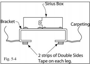
(d) Remove the 2 release tabs from the bottom of the bracket and mount the bracket to the floor pan. (Fig. 5-4 & 5-5)
