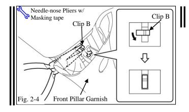
(3) Using tape-wrapped (to prevent damage) needle-nose pliers, rotate clip B 90°. (Fig. 2-4)
