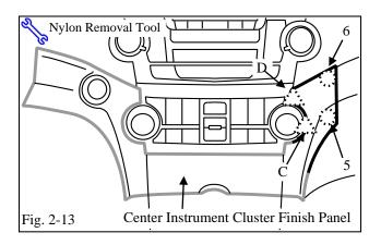
(3) Using a Nylon Removal Tool, disengage Clip 5 and 6, and Claw C and D. (Fig. 2-13)
